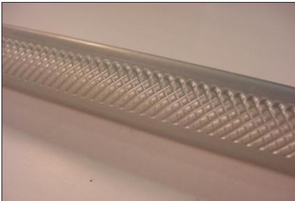
Figure 8: Thermoplastic Pultrusion Tool Handles – Inline Capstock Knurling
