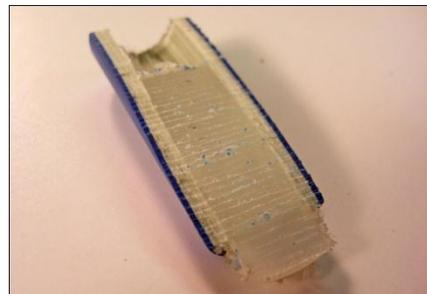
Figure 12: Spin Welding of End Plug into Thermoplastic Pultrusion Tool Handle
