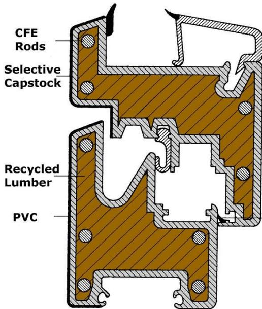
Figure 15: Selective Reinforcement Concept (5)
