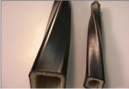
Figure 13: Post Forming of Thermoplastic Pultrusion - Twisting
