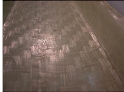
Figure 10: Transverse Fiber Thermoplastic Pultrusion Channel profile – no capstock
