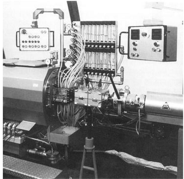
Figure 4B Vacuum tank with short vacuum calibration unit for profile and pipe production (8) p. 94
