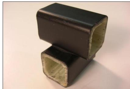
Figure 11: Thermal Part Welding of Thermoplastic Pultrusion
