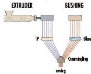
Figure 3: Commingled glass/polypropylene fiber manufacturing process.
