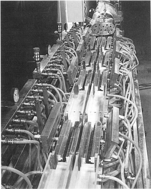
Figure 4 Twin orifice die and vacuum block calibrator used in window profile extrusion (8) p 89
