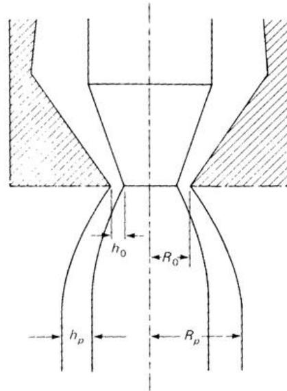
Figure 1: Die Swell behavior of extruded tubular profile. (6) p. 473
