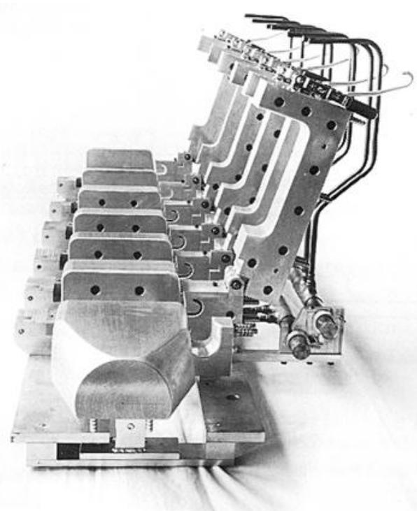
Figure 4A Extrusion segmented or template calibration (8) p. 91
